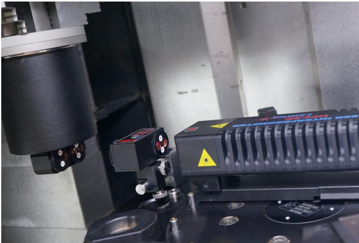
FIG.14.2. OPTICAL PATH SET UP FOR ANGULAR POSITIONING MEASUREMENTS-PHOTO
