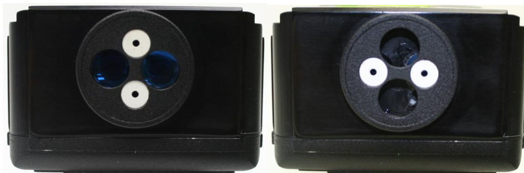
FIG.4.4. DIAPHRAGM POSITIONS. A) MEASUREMENT, B) ALIGNMENT
