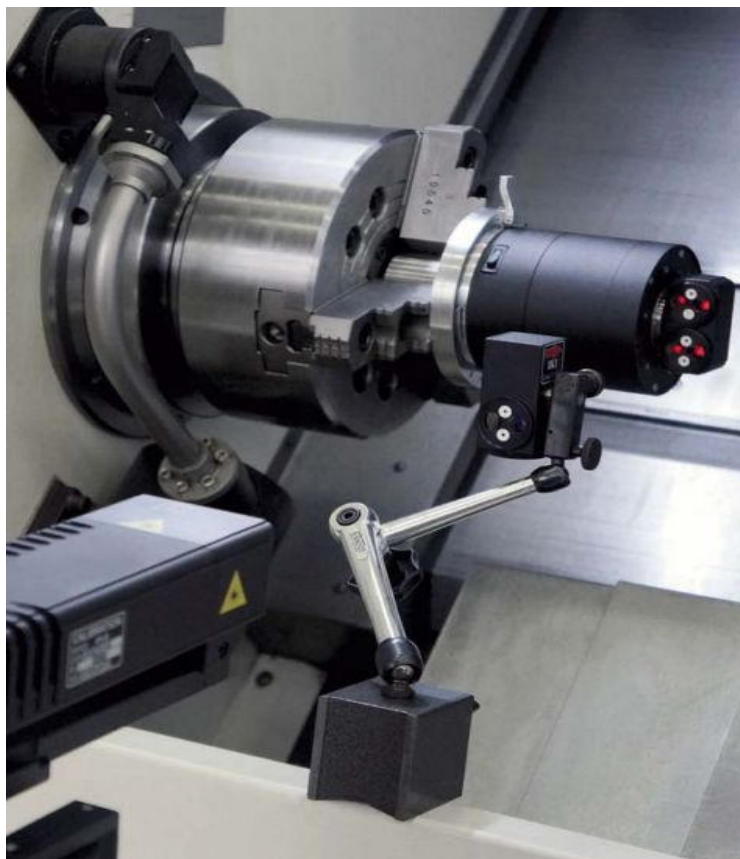
FIG.14.2. OPTICAL PATH SET UP FOR ANGULAR POSITIONING MEASUREMENTS- PHOTO
