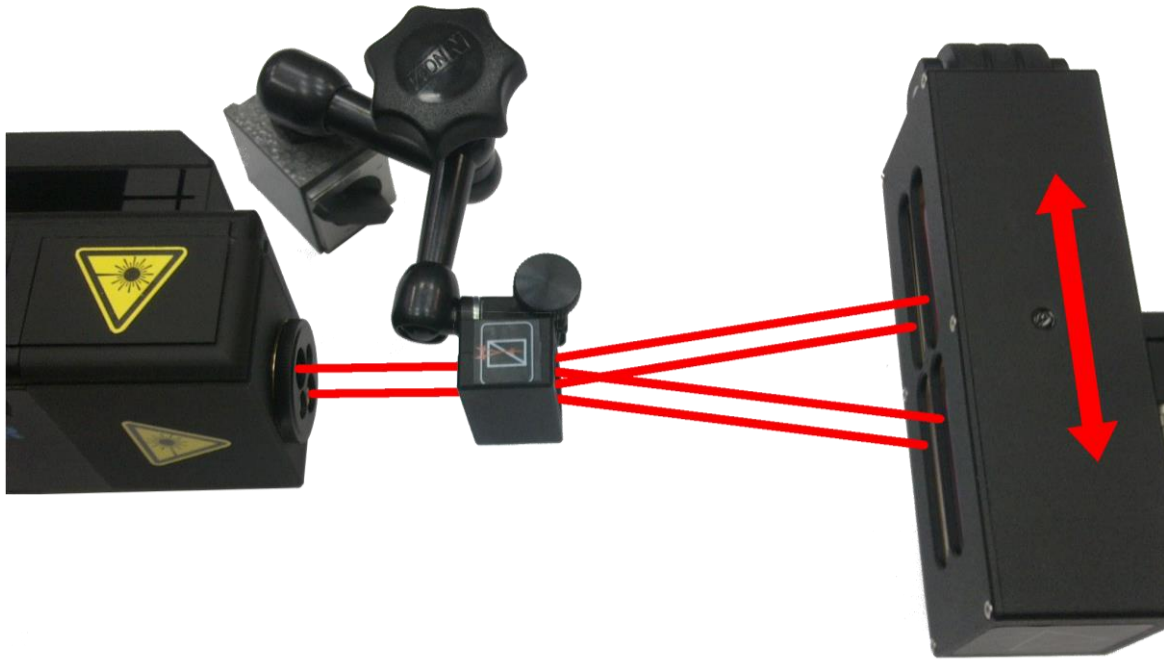
FIG.7.16 OPTICAL PATH SET UP FOR WOLLASTON STRAIGHTNESS MEASUREMENTS IN Z AXIS.
