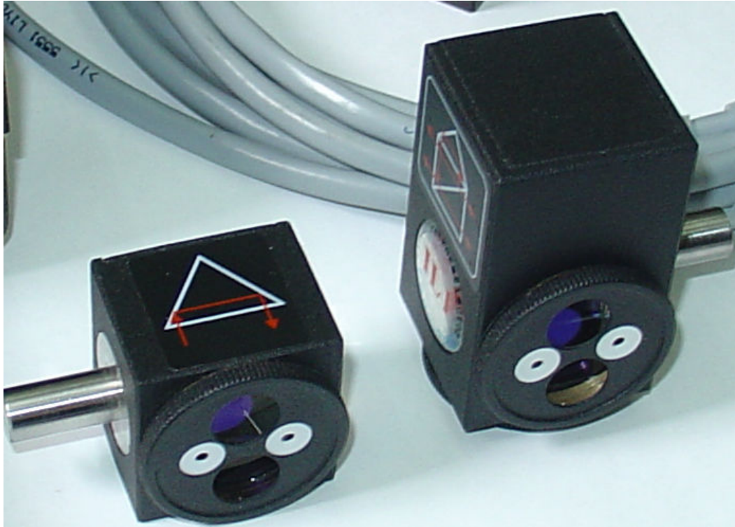
Fig. 3.4. Reflector RL1 and interferometer IL1 with diaphragms set into work position.
