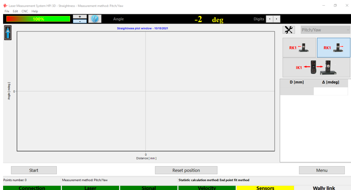
FIG.16.5. PITCH/YAW MEASUREMENT WINDOW.
