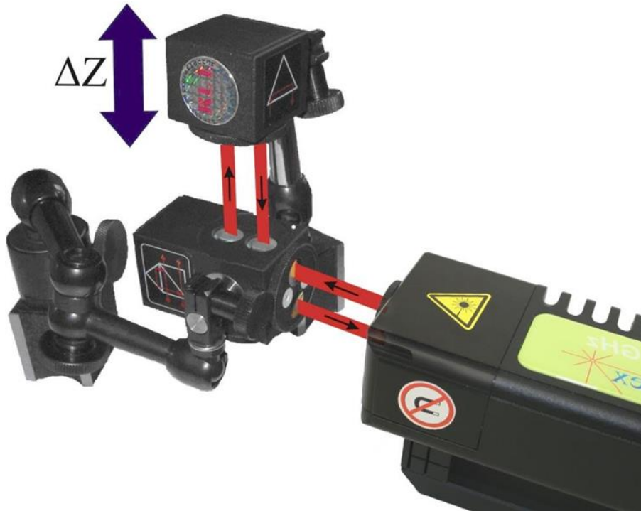
FIG.13.4. OPTICAL PATH SET UP FOR LINEAR DYNAMIC MEASUREMENTS IN Z AXIS
