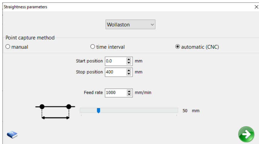
FIG.9.39. SELECTION OF CONFIGURATION OF THE WOLLASTON OPTICS
