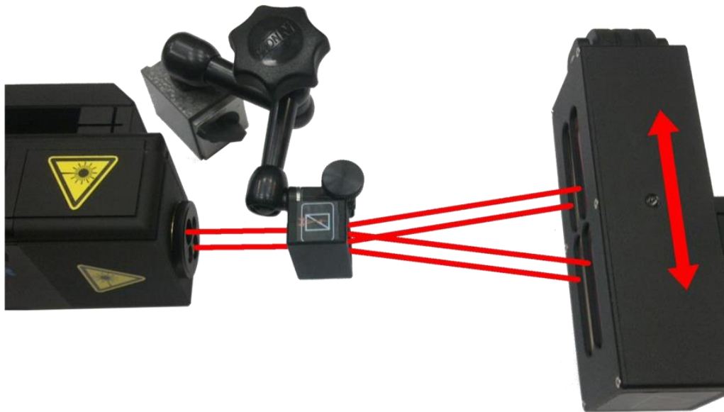
FIG.7.15 OPTICAL PATH SET UP FOR WOLLASTON STRAIGHTNESS MEASUREMENTS IN Z AXIS.
