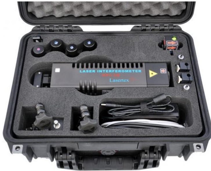
FIG.3.19. THE SUITCASE FOR TRANSPORT AND STORAGE OF THE INTERFEROMETER SYSTEM.
