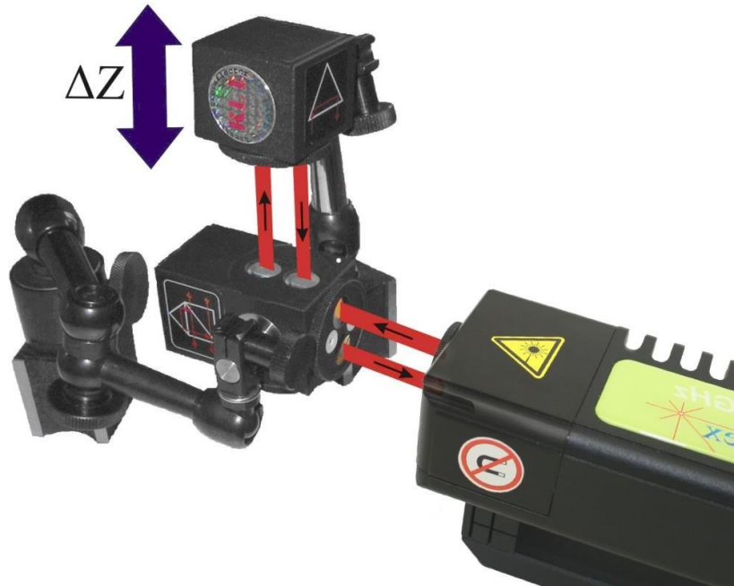
FIG.15.3. OPTICAL PATH SET UP FOR VELOCITY MEASUREMENTS IN Z AXIS.
