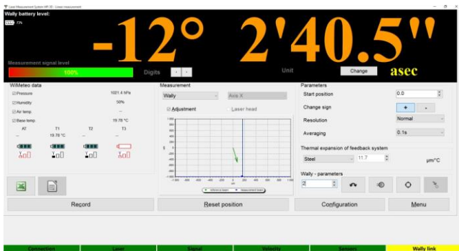
FIG.14.11. DISPLAY WINDOW WHEN ROTARY ENCODER IS PRESENT
