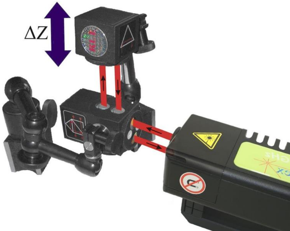
FIG.12.4. OPTICAL PATH SET UP FOR VIBRATION MEASUREMENTS IN Z AXIS
