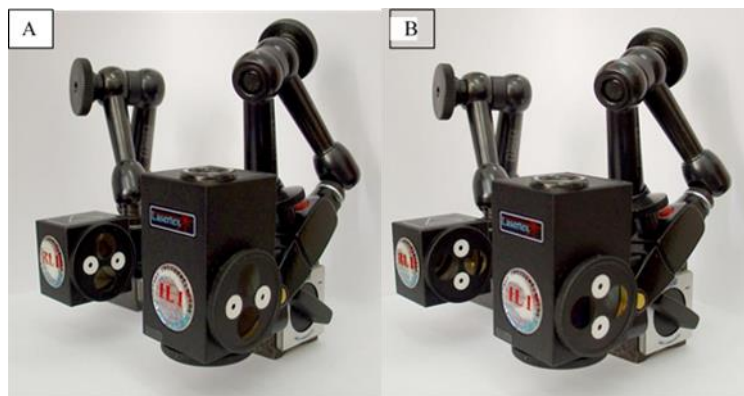
FIG.4.5. DAPHRAGMS: ALIGNMENT POSITION (A) AND WORK POSITION (B)
