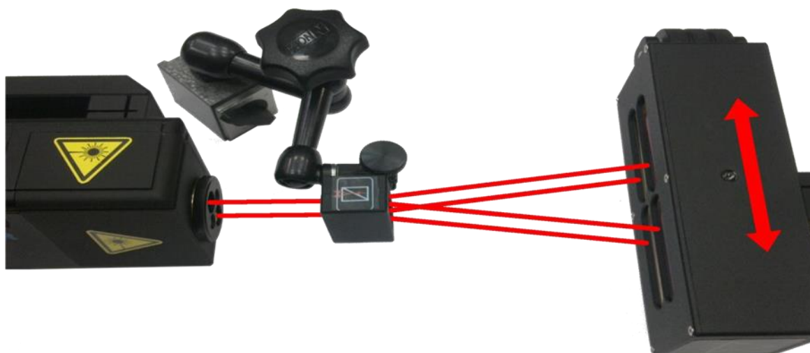
FIG.13.11. OPTICAL PATH SET UP FOR DYNAMIC STRAIGHTNESS MEASUREMENTS IN Z AXIS
