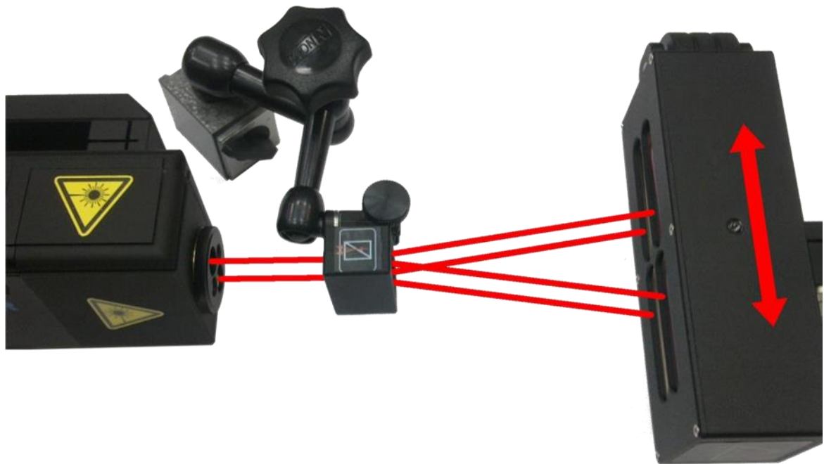
FIG.7.16 OPTICAL PATH SET UP FOR WOLLASTON DYNAMIC STRAIGHTNESS MEASUREMENTS IN Z AXIS.
