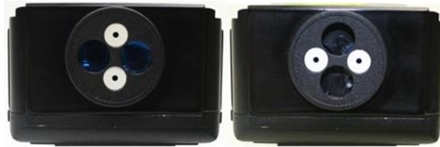
FIG.4.4. DIAPHRAGM POSITIONS. A) MEASUREMENT, B) ALIGNMENT
