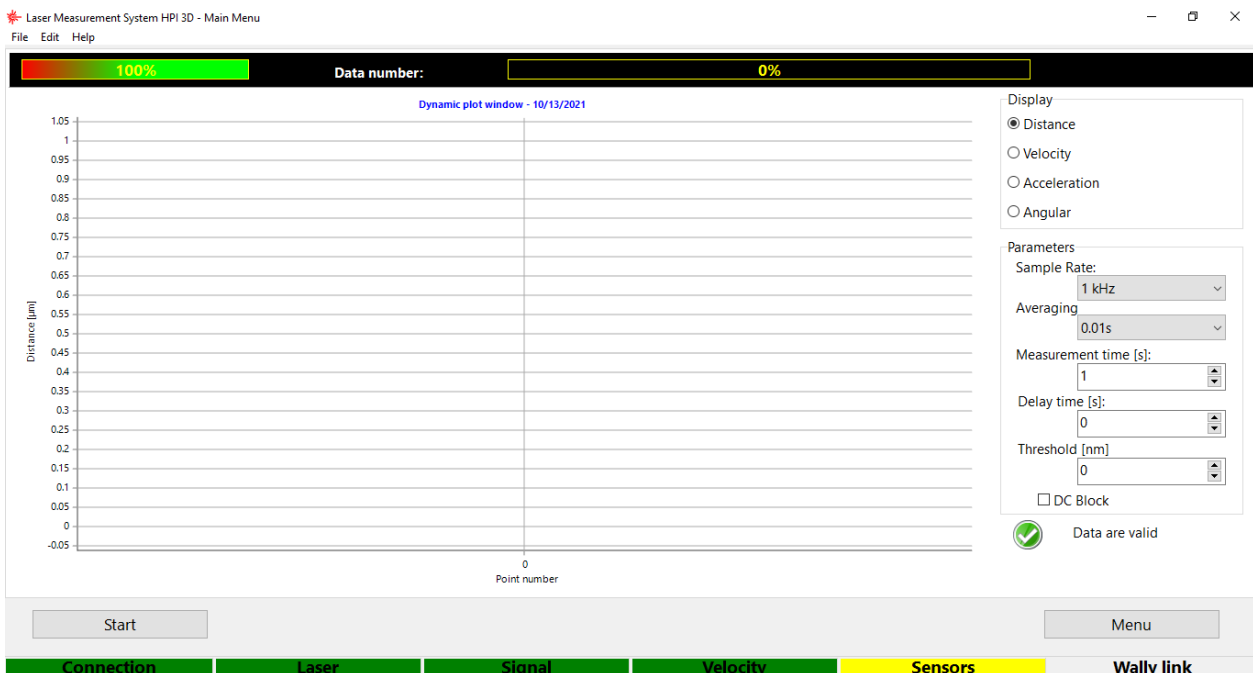
FIG.13.12. DYNAMIC MEASUREMENT WINDOW
