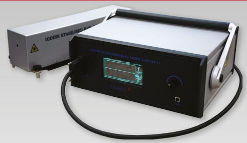
Frequency Laser Standard is automatic laboratory device designed to compare and calibrate He-Ne (632,8nm wavelenght) lasers. Absolute laser frequency is defined by iodine vapour cell. This is unique laboratory device with automatic absorption peaks detection and results presentation on graphic display.
