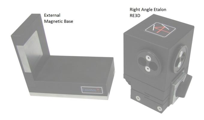
**Right Angle Etalon RE3D** can be used to measure squareness in the same plane as a laser head base or in perpendicular plane to the laser head using external magnetic base. Thanks to the special set of inside mirrors the output beam, is always reflected at 90° according to the incident beam. As long as you place all Lasertex elements at the same plane you don't have to adjust their hight, we made it for you. We recommend you to set Right Angle Etalon RE3D after the Linear Interferotemer IL1.
